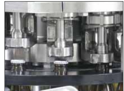
Plain bearing bushes made of ZX-100K in a beverage filling machine. Polyamide was substituted.
