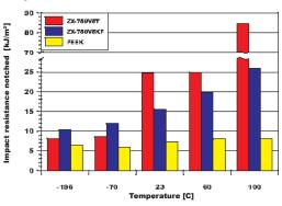
ZX-750V5T has got a 500 % better Charpy v-notch test value than PEEK (at 23 °C). The fibre reiforced ZX-750V5KF is more impact resistant than natural PEEK.
