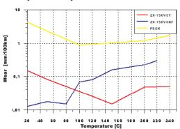
So far, from 100 °C, the ZX-750V5T offers the best measured wear resistance. ZX-750V5T is from 2000 % to 8000 % more wear resistant than PEEK (natural).
