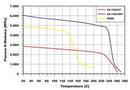
The elastic modulus of both ZX-750 types, strongly decrease over 220 °C. This decay temperature is 80 °C higher than the PEEK's one.
