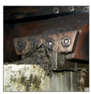
The existing sliding guide of a chipboard press, is converted from a grease lubrication condition to a dry running condition. Thanks to the extreme high PV-value and the high wear resistance of the ZX-750V5T, the chipboard press now works just in dry running conditions.
