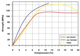
ZX-750V5T does have a similar behaviour to PEEK up to a pressure of approx. 100MPa. ZX-750V5KF is stiffer and its compression at break is approx. 11%.
