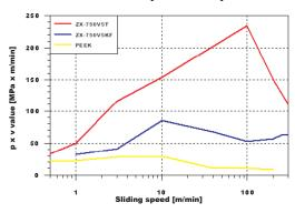
The PV-value of the ZX-750V5T is 1000% higher than the PEEK's one. PEEK in combination with a oil lubrication has got lower resistance.
