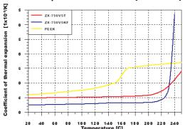
The thermal expansion coefficient of the ZX-750V5KF is up to  $220\,^{\circ}\text{C}$  at the same level of aluminium.
