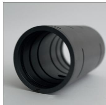
ZX-530CD3 is used as piston guides in pneumatic cylinders. Thanks to the very low wear and low thermal expansion a very tight clearance is possible.
