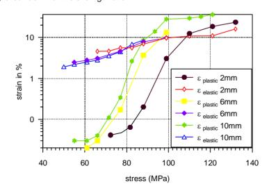
III. 2: elastic and plastic deformations of ZEDEX 100K exposed to stress (60s) of different material thicknesses
